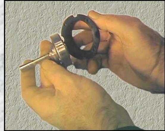
After removing the large 'C' ring from the propeller shaft support the bearing by the inner race in a suitable vice, using a nylon rod and small hammer, gently tap the shaft through the bearing.
