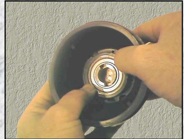
Secure the bearing housing into the casing, use four long shank round head No.1 Philip's screws with four small flat washers.
