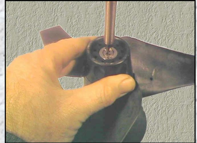
Final checks can now be carried out. Ensure the blades spin freely. Check the operation of the pitch setting knob.
