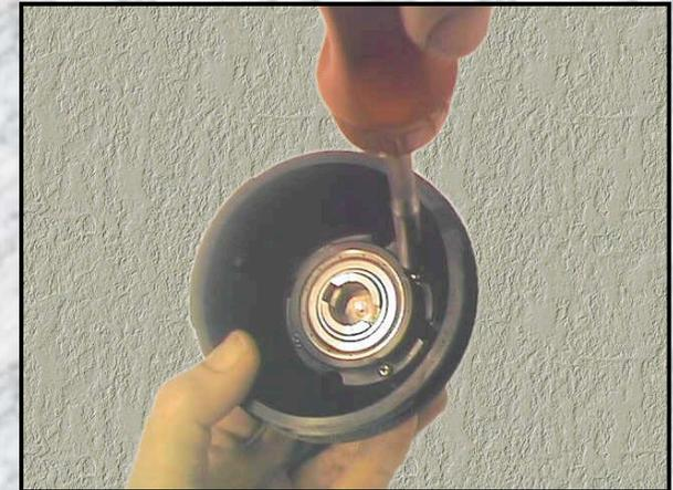
The propeller shaft and bearing should now be secure. Test for smooth rotation by spinning the shaft, if using old bearings check carefully for any binding.
