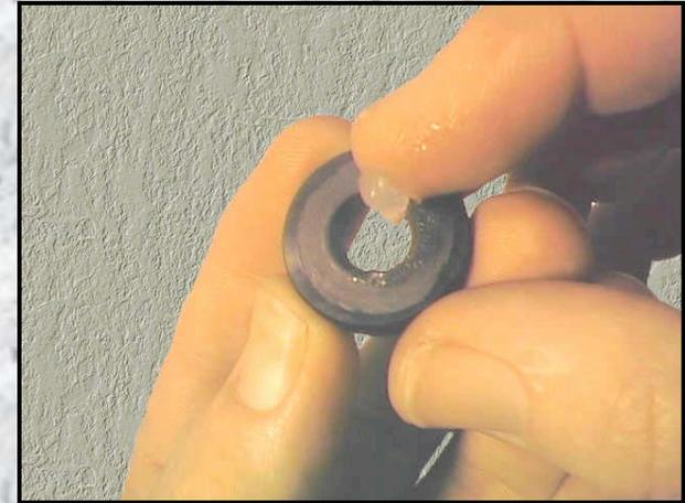
Lubricate the FA seal with silicone grease. Smear the lubrication on the opposite side to the spring, this will ensure the knife edge has lubrication after being installed.
