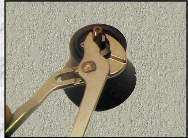
Turn the housing over to gain access to the four screws that secure the large bearing housing. Remove these screws and washers.
