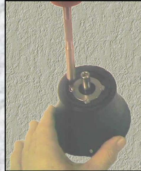
Line up the drive pin holes in the shaft with the slots in the casing and install the drive pin. Ensure the pin is centred.
