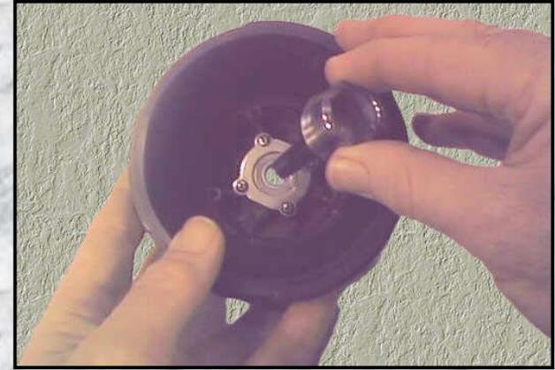
The large bearing is now pressed by hand into the bearing housing.
