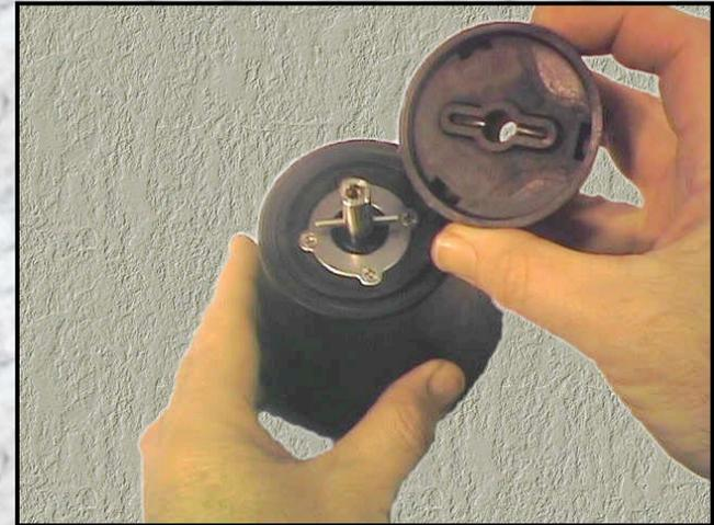
The clutch screw assembly is now fitted. The star washer sits on the boss first, next the spring cup washer, the inner edge should sit on the star washer and the outer edge is curved up.
