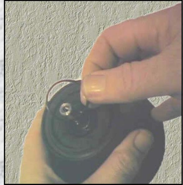
Ensure the o ring is in position, fit the bearing retainer. The countersunk holes in the retainer face up.
