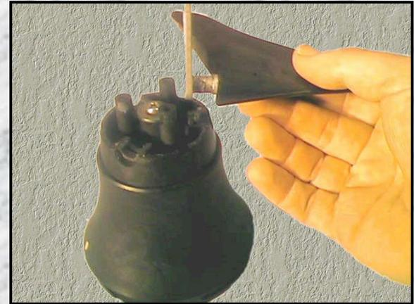
A No.3 Philip's screw driver is required to undo the centre screw from the propeller base.
