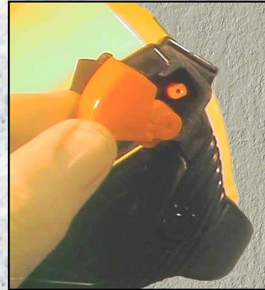
Fit the retaining screw and spring sleeve. Do not over tighten the screw - it is secured into a plastic thread.
