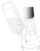
**Refill with one-way valve** between dives. It is no longer necessary to detach the cap for refill of wick between dives. Always detach the first stage from tank prior to adding water. Insert nozzle of fill bottle into valve opening. Special tip will automatically open valve and allow filling. Each Mark is a unit. Use 1.5 - 2.5 units per refill.
