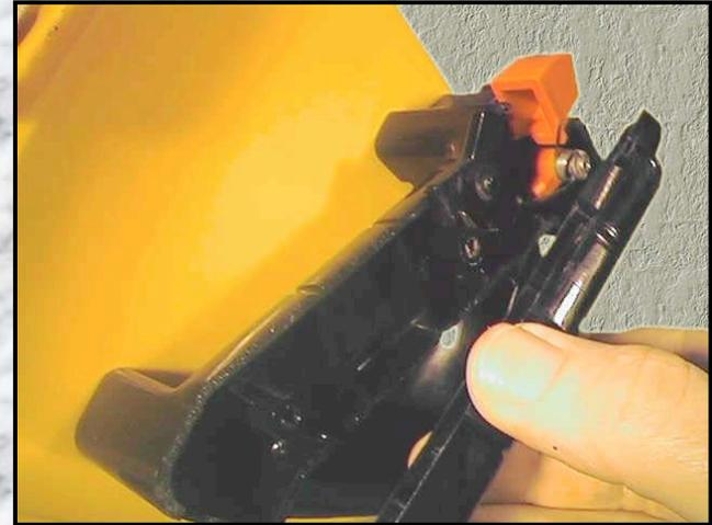
Note the position of the spring before removing, this could help with refitting. Remove the button retaining screw together with the spring and metal sleeve.
