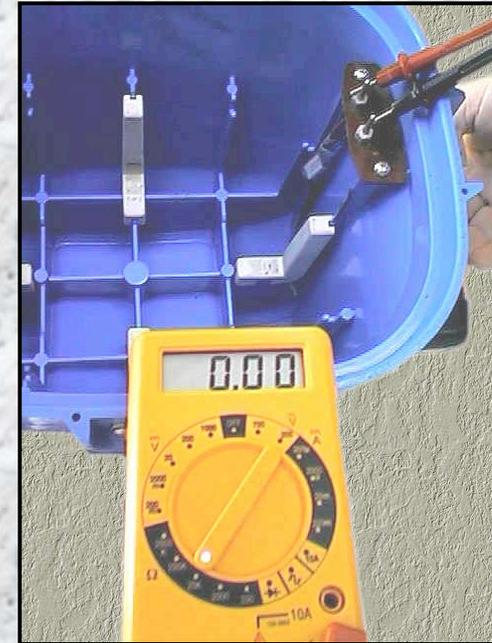
The reed switch is glued to the front cover with contact cement.
